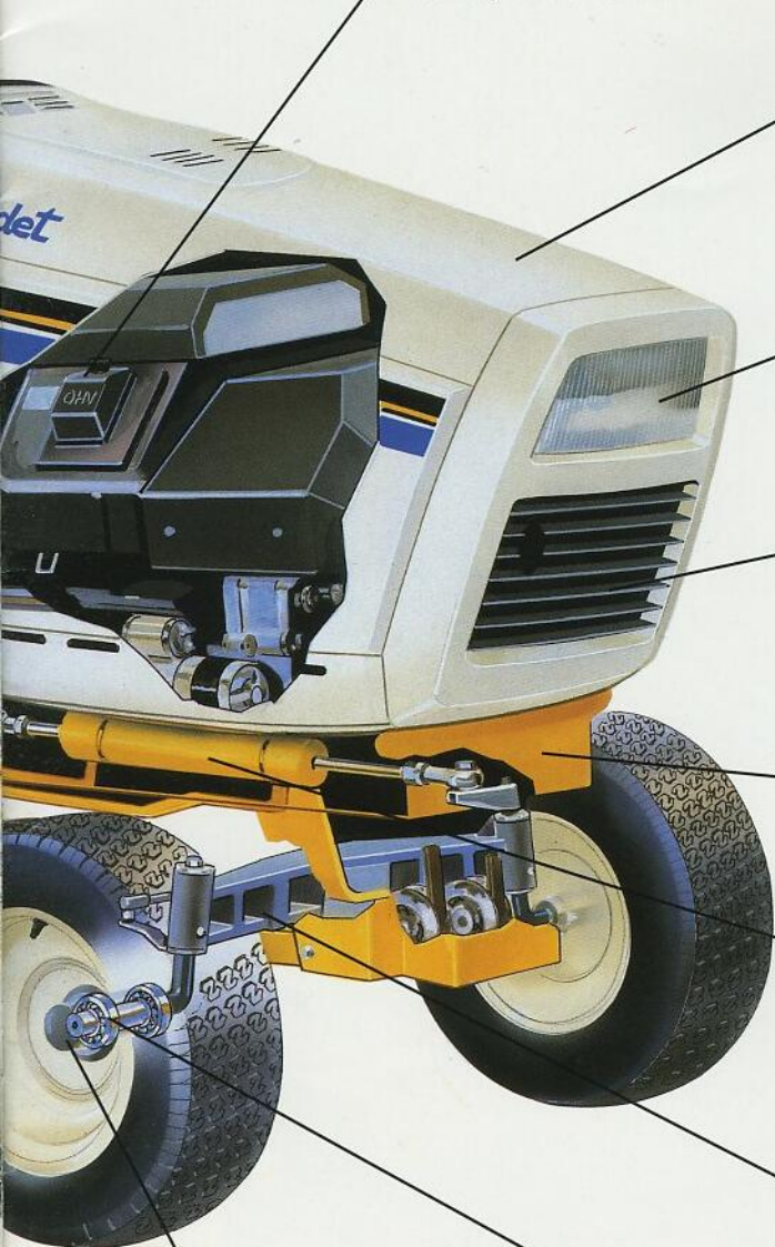
OHV V-twin cylinder engine with full-pressure lubrication and spin-on oil filter
