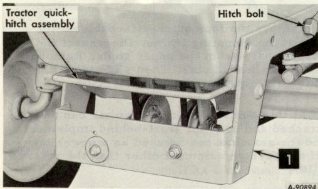
Illust. 8A Mounting on Cub Cadet 72, 104, 105, 124, and 125 Tractors.
