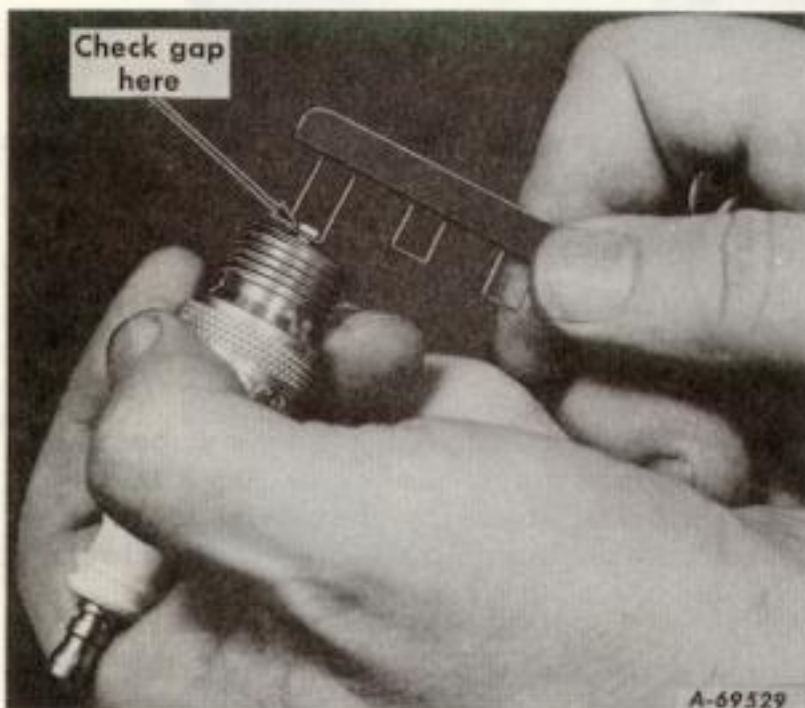
Illustr. 17 Checking the spark plug gap. Set gap at .025-inch.
