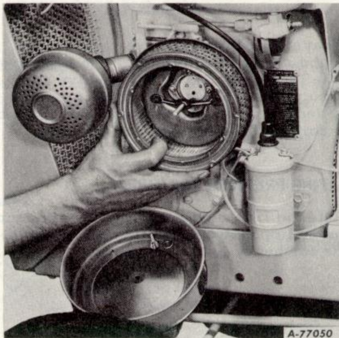
Illust. 15 Removing the air cleaner filter element.
