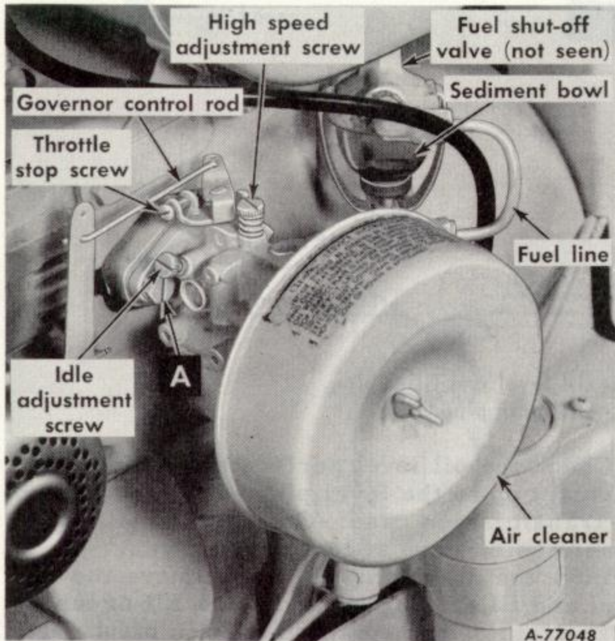
Illust. 14 Carburetor and fuel strainer. (Seven horsepower engine.)
