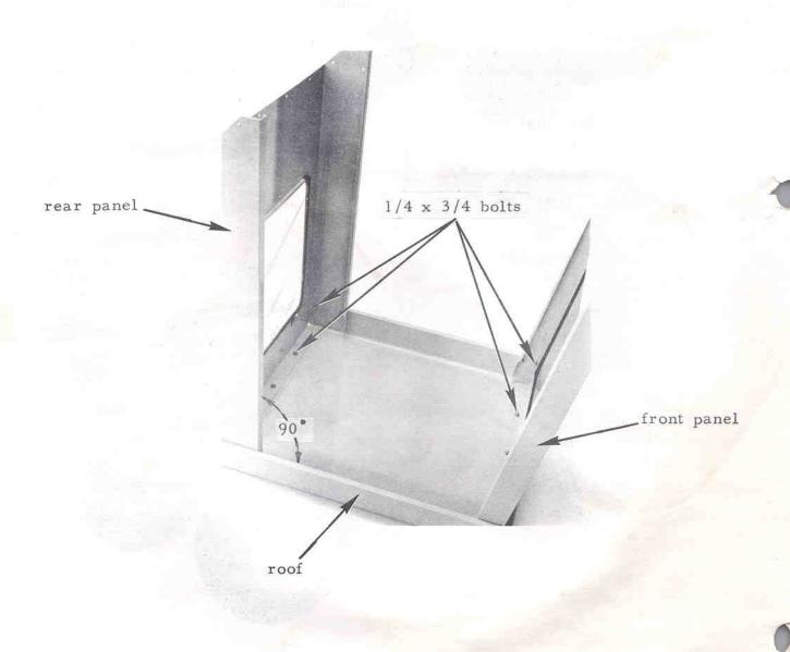
2. Attach catches, lower rear panel, front mounts and rear mounts L.H. & R.H. using 1/4 x 3/4 hex head bolts, flat washers, lockwashers and nuts. Insert 3/16 x 3/4 screws into hole in front edges of rear and front panels, fasten into position using 3/16 nuts.
