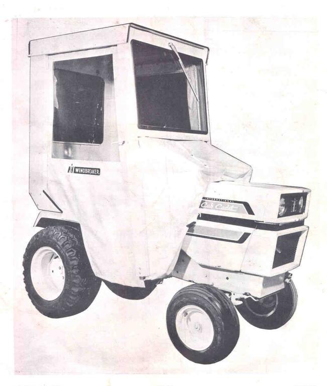
1. Fasten front and rear panels to roof using 1/4 x 3/4 hex head bolts, flat washers, lockwashers and nuts. Fully tighten rear panel after squaring it with roof, hand tighten front panel.
