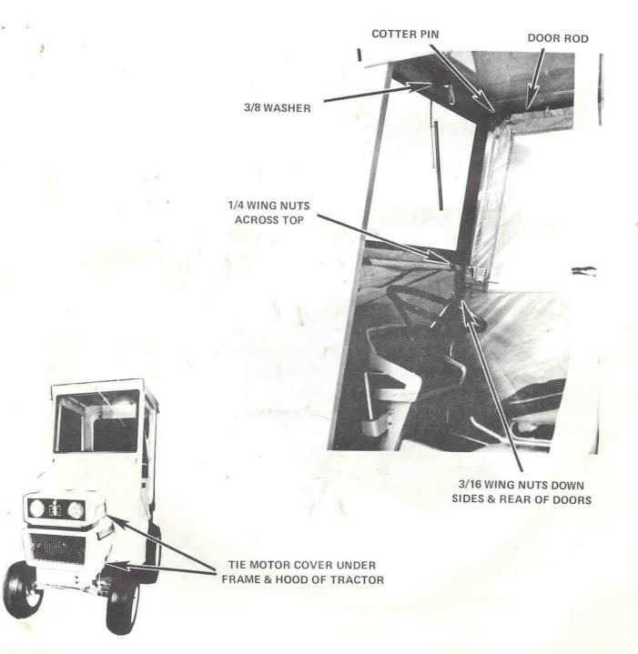
6. Close doors and pull rear panel back until slack is taken up in doors. (Check clearance between rear panel and seat by tilting seat.) Back drill 9/32 diameter (.281) holes in fenders through rear mounts. Use 1/4 x 1 hex head bolts, largewashers, flat washers, lockwashers and nuts.
