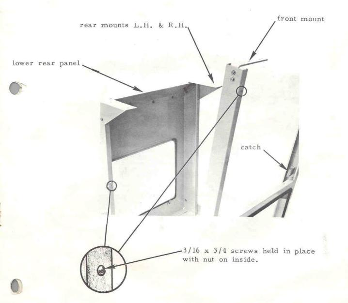
3. Remove slotted screws from front of foot rests. Position cab on tractor and fasten front mounts to foot rests with motor cover supports in position using 5/16 x 1 hex head bolts, flat washers and lockwashers. Cut vinyl molding to length and glue to front and back edges of roof, rear window opening and rear mounts.
