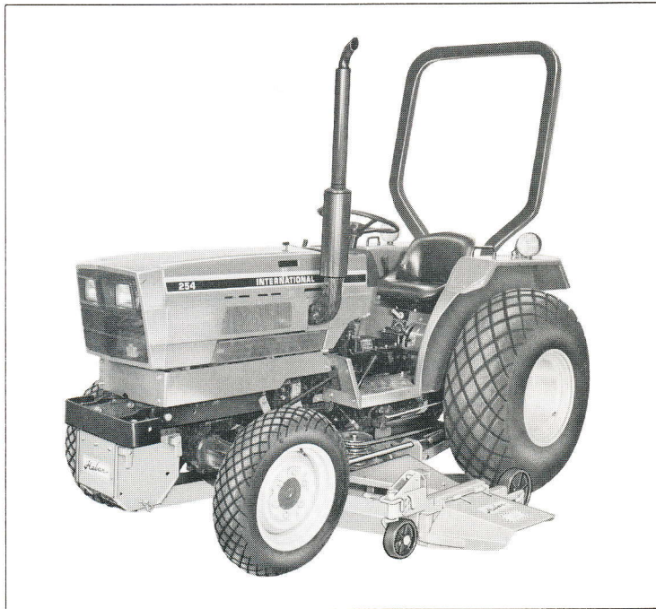
MODEL 254 INTERNATIONAL HARVESTER TRACTOR WITH 616-IH61 61" CUT MOWER-REAR PTO DRIVE.
