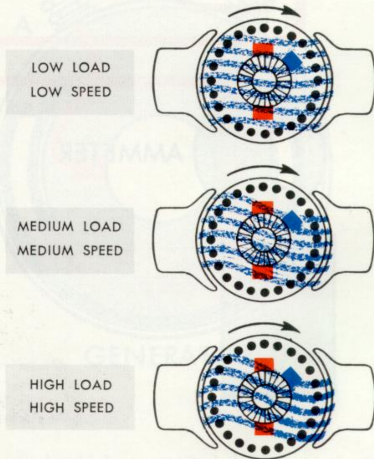
Illust. 80—Showing armature reaction at different speed of third brush generator.
