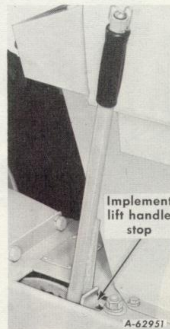
Illust. 10B Adjustable stop limiting handle travel.
