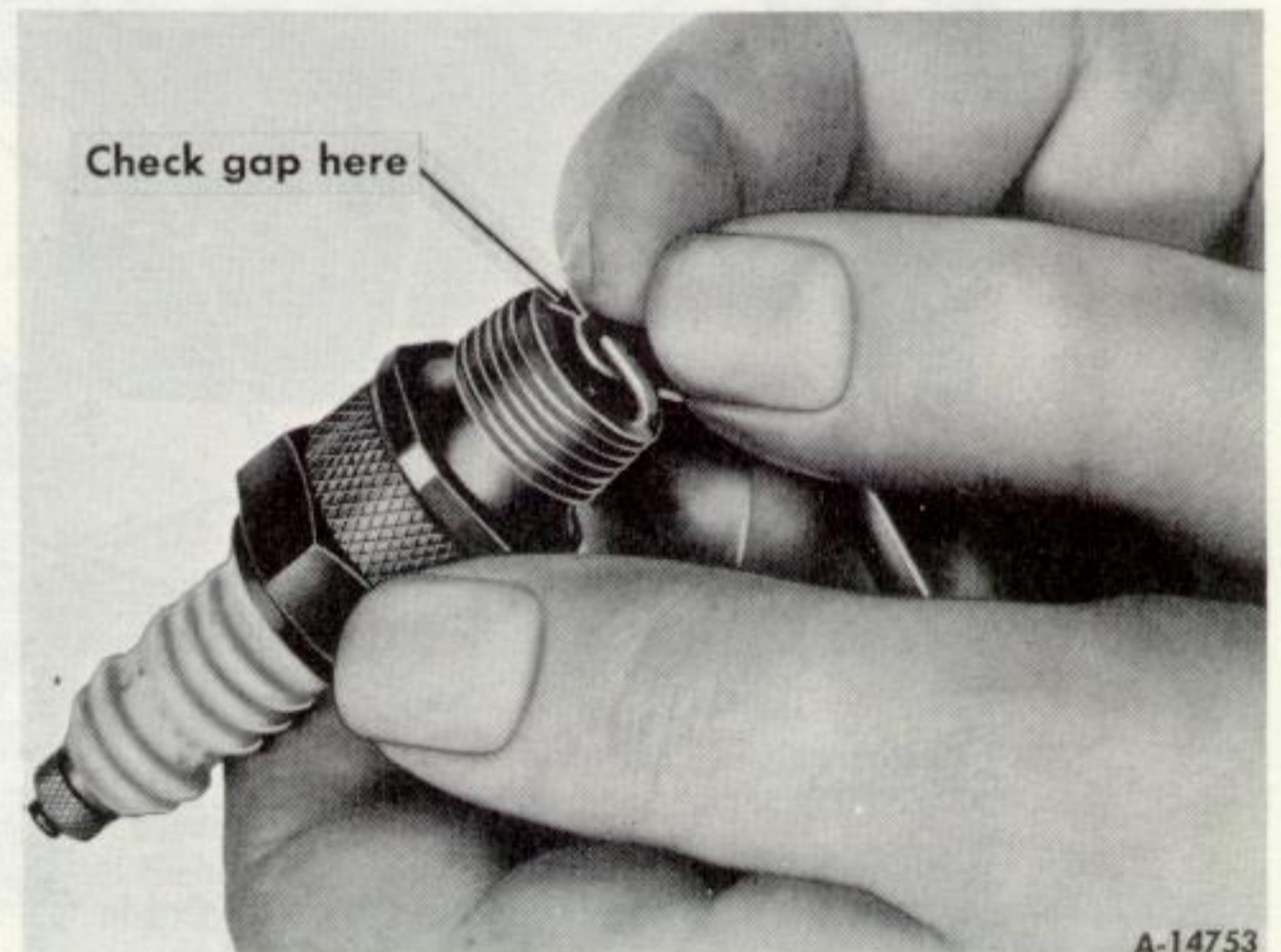
Illust. 21A Checking the spark plug gap. Set gap at .025 inch.
