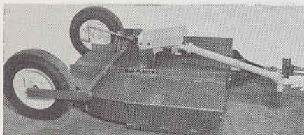
Reversible Axle -- Standard Use Wheels Side or Rear
