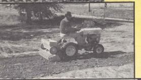
With scarifier attachment you can rip up hard packed ground. Additional down pressure caused by scarifying teeth help Grid Roller pulverize clods.
