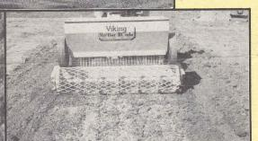
When grade is established, fertilizer and/ or seed can be spread with precision.
